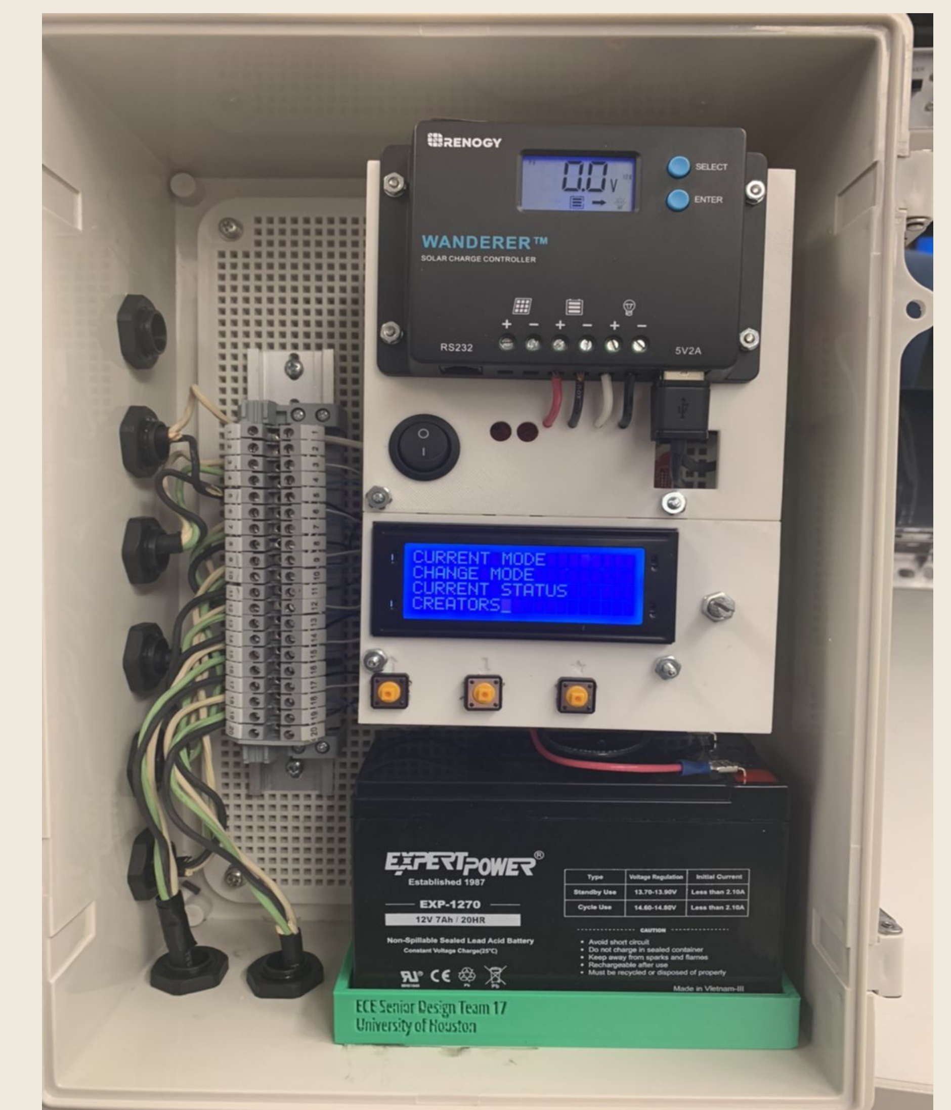
Figure 4: Inside the SDIS, with the battery, shield, charge controller, LCD, and interactive components displayed
